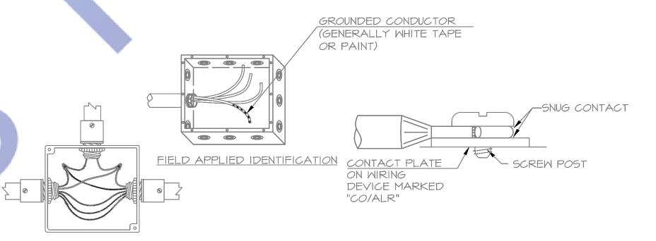
TYPICAL CONNECTION OF WIRES IN JUNCTION BOX
